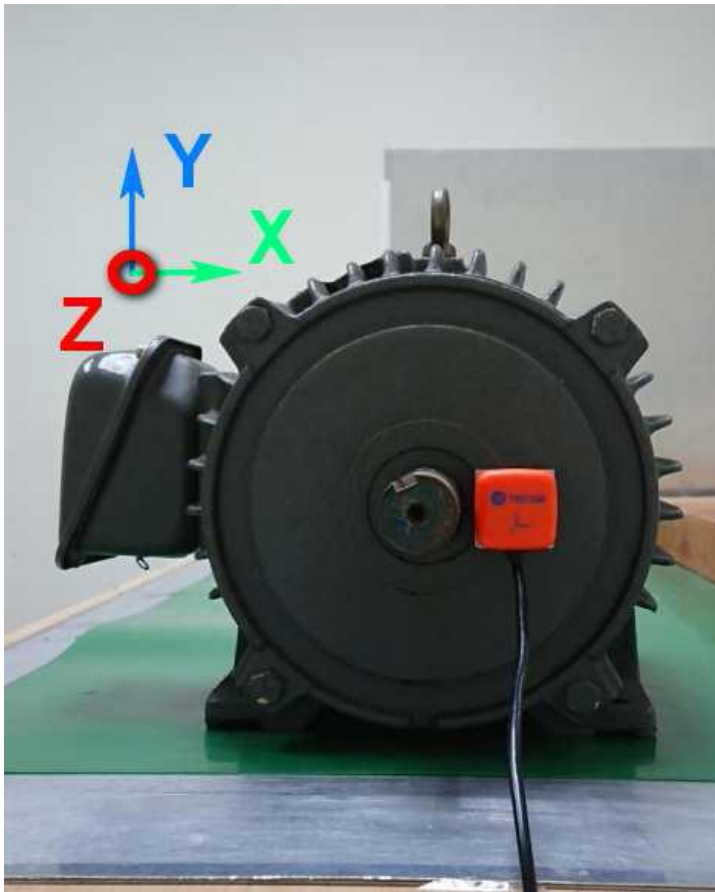
When using the axial installation position, the figure represents the measured correct vibration axis.
