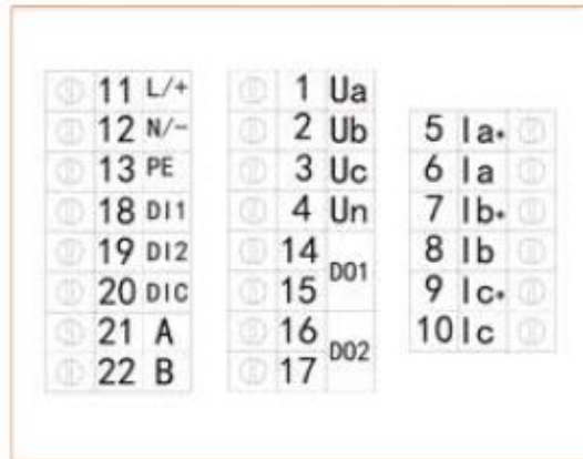
The Pin Assignment of Terminal
